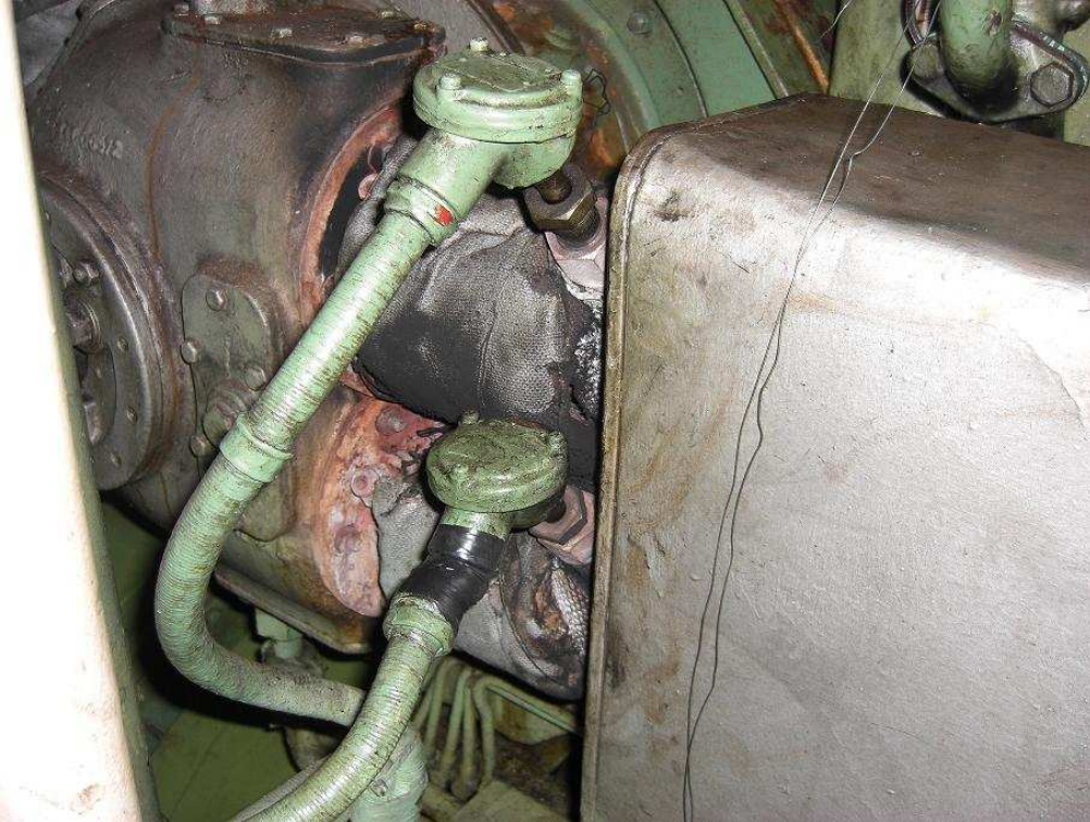
MV Dorothea: corrosion at superstructure, insufficient insulation of hot surfaces in engine room, etc.
