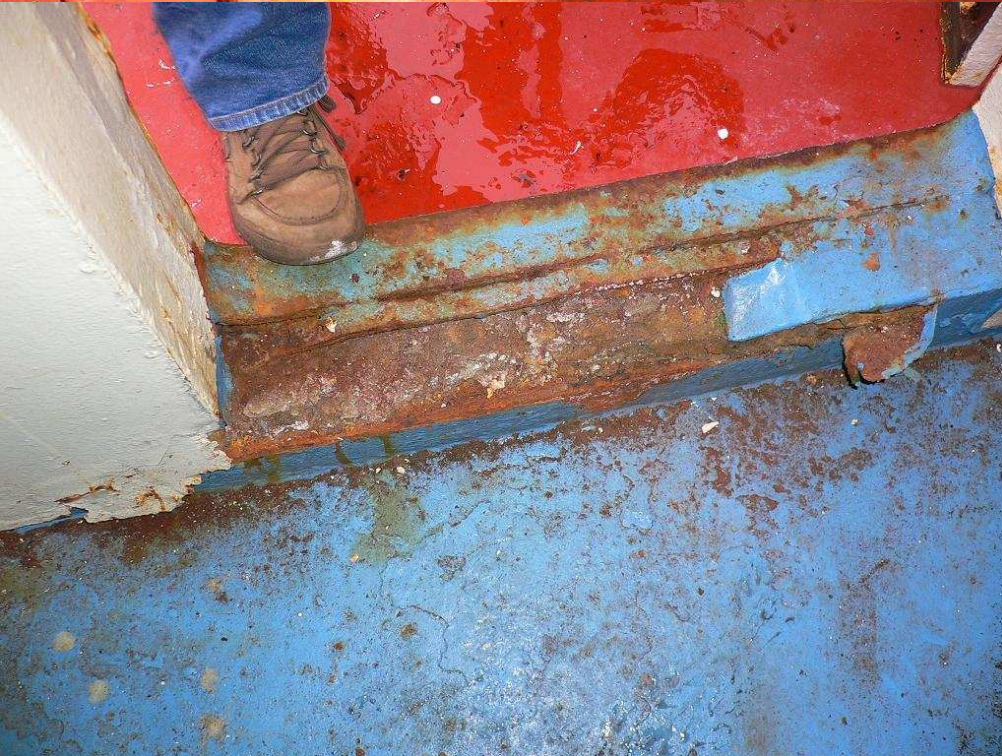
MV Reksnes: poor maintenance, corrosion, cracks, missing gear wheel protection, etc.
