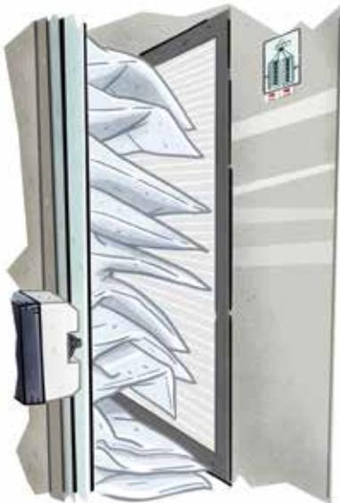
After a long period of operation, air filters are known to be microbially contaminated. When removing contaminated filters, bacteria, moulds, endotoxins, etc. can be expected in addition to heavy dust formation. This is especially true for vessels that have dust-forming cargoes, e.g. grain as bulk goods. Therefore, protective measures must always be taken when replacing the air filter.
