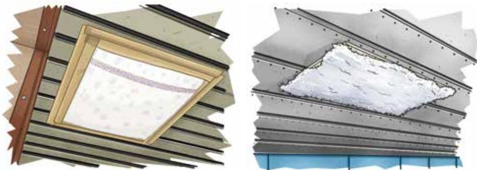
Fig. 10: Supply air terminal unit with wiping cloth (left) respectively supply air terminal unit with filter material (right)
